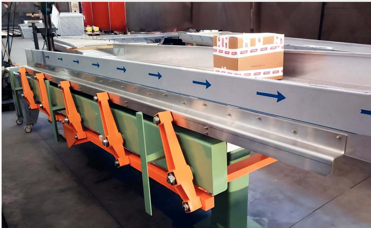
Oscillating Mountings: AD-P – Double Rocker (Customized Design)
