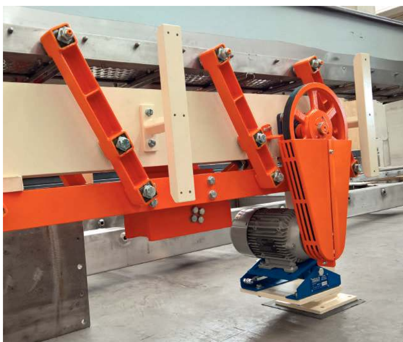
Oscillating Mountings: AD-P – Double Rocker (Customized Design)
